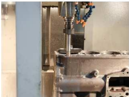
Illustration 161 Lifter clip spring guide bore on 9.3L C9. Lifter clip spring guide bores next to lifter bores that are sleeved cannot be repaired as there will not be enough material between the two bores.
