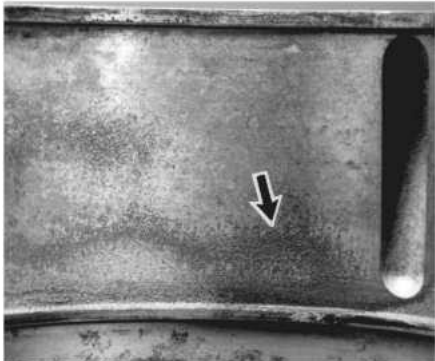
Illustration 78 g06344278 Erosion damage showing signs of early problems in the cooling system.
