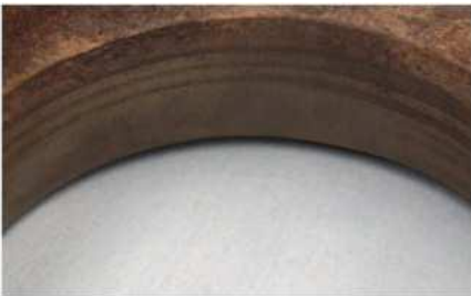
Illustration 118 g06238807 Erosion in the lower cylinder bore
