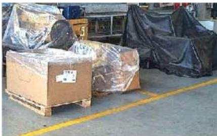
Illustration 232 g06278539 Example of protection for a component that is stored for a longer period
