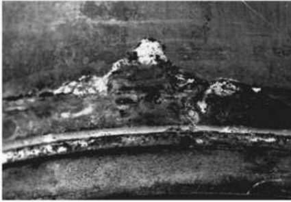
Illustration 77 g06344272 Corrosion which occurred during engine storage.
