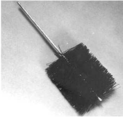
Illustration 47 g06338340 Typical example of a nylon brush that is used to clean the cylinder bores
