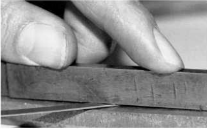
Illustration 65 g01531335 The spacer plate is bent or warped.
