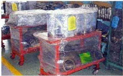
Illustration 231 g06278538 Example of protection for a component that is stored for a shorter term
