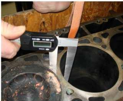
Illustration 51 g01360198 Measuring cylinder bore wall thickness with 93028 Digital Disc Brake Caliper
