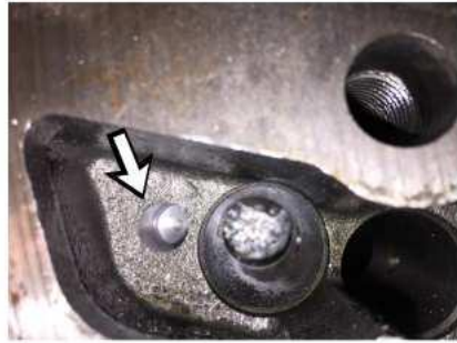
Illustration 161 Lifter clip spring guide bore on 9.3L C9. Lifter clip spring guide bores next to lifter bores that are sleeved cannot be repaired as there will not be enough material between the two bores.
