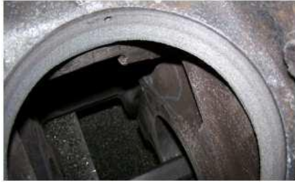
Illustration 122 g06238797 Lower liner bore machined with step remaining.
