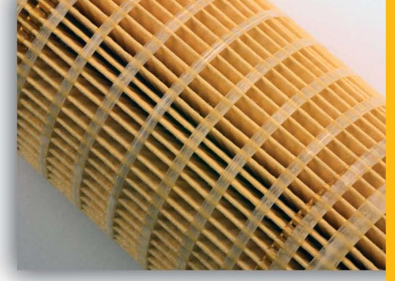
Cat<sup>®</sup> Filters have a fiberglass cord wrapped around the cylinder of filter media. This spiral roving keeps pleats in place, allowing for better filtration.
