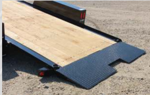
Long approach ramp allows easy equipment loading and unloading.
