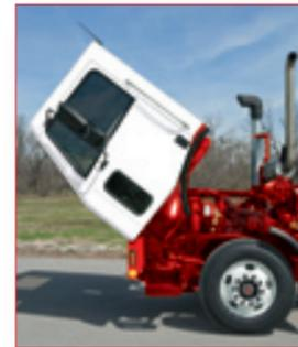
Cab Tilt for Engine Access
